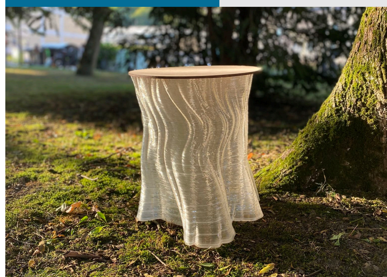
Procedural design seat made from PLA; "Wandering Factory"; AEC Festival 2021; Cooperation with Creative Robotics, Univ. of Arts Linz
